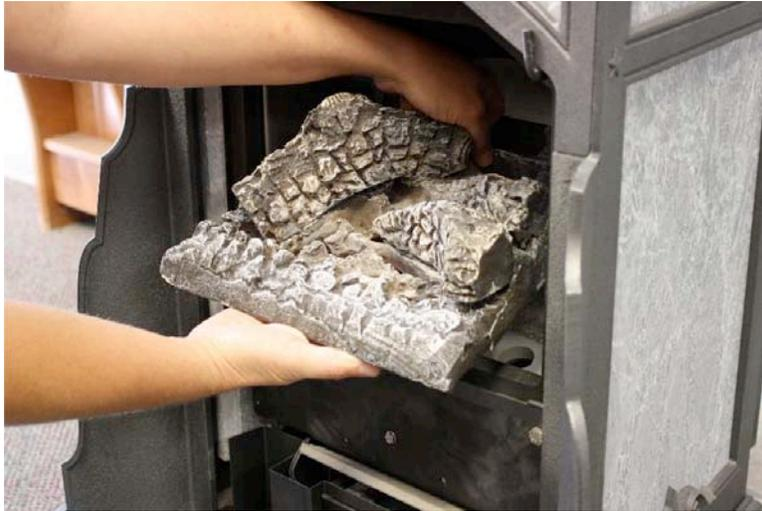
7. Now pull the original tile off the top surface of the burner pan.
