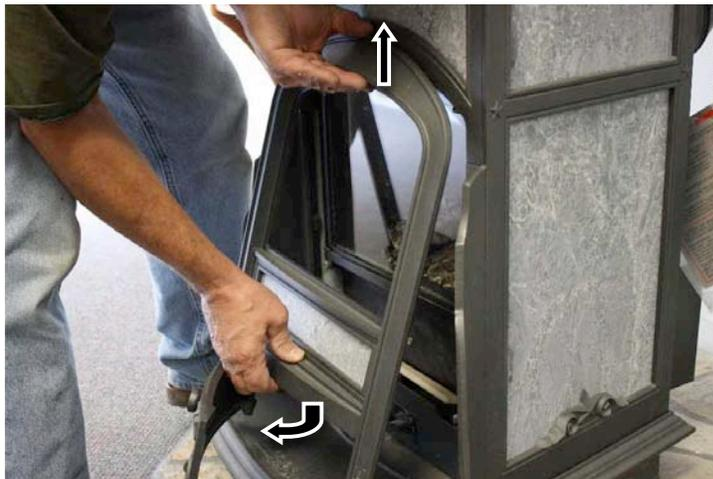
3. Use pair of pliers or the window clip tool that came with your stove to release the two window clips. Pull them out and twist them out of the way.
