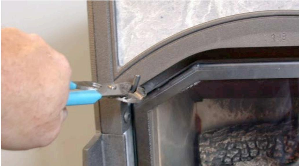
4. Remove the glass window and frame assembly by pulling the window up out of the bottom glass retainer and out away from the stove.
